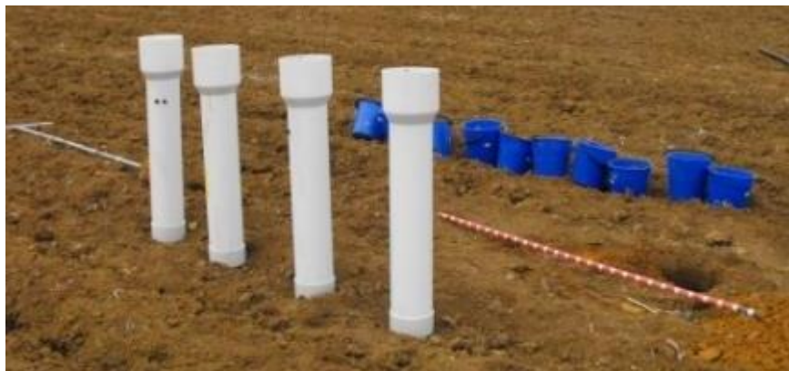
Figure 1. Basic passive wick tension fluxmeter design installed at all sites. The units are installed below the soil surface, and intercept drainage water and hold it in a storage tank until sampling. Diatomaceous earth and fine sand are packed into the convergence zone to filter drainage water. The maximum storage volume is about 14 L.
