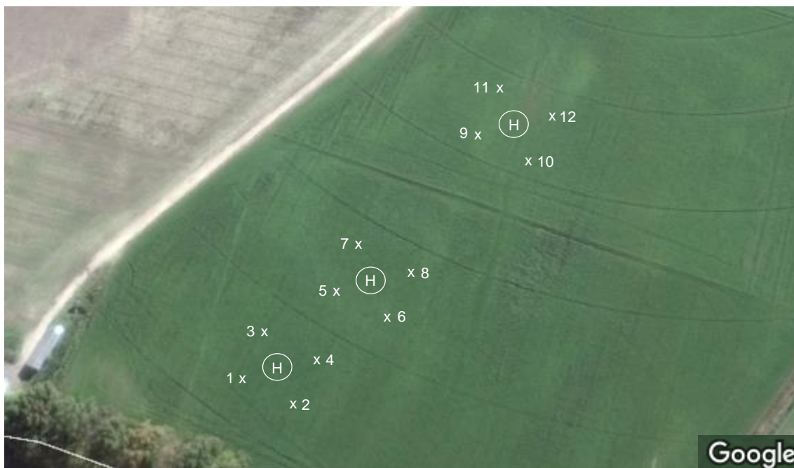
Figure 2. Example layout of fluxmeter units within a field. Clusters of four units were installed within a 4 m radius and tubing was trenched back to a central sampling hub (H). The distance between clusters depended on site features and ranged from 25 to 40 m.
