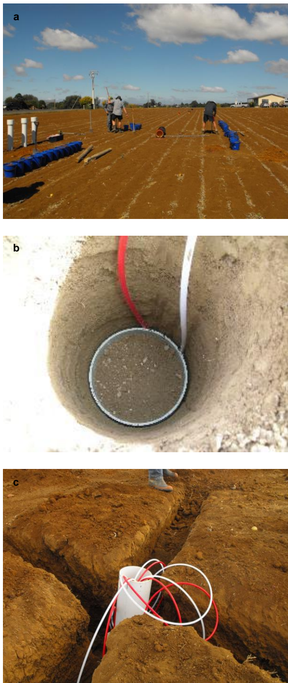
Figure 3. Example of the installation process showing (a) preparation of the holes for installation and soil being hand-augered into buckets according to depth, (b) lowering of the fluxmeters into holes, and (c) tubing coming from the individual fluxmeters back to central hub sampling points.
