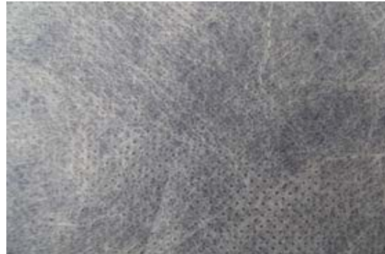
(b) Light reduction cloth used to shade plots, lowering light levels by 30%.
