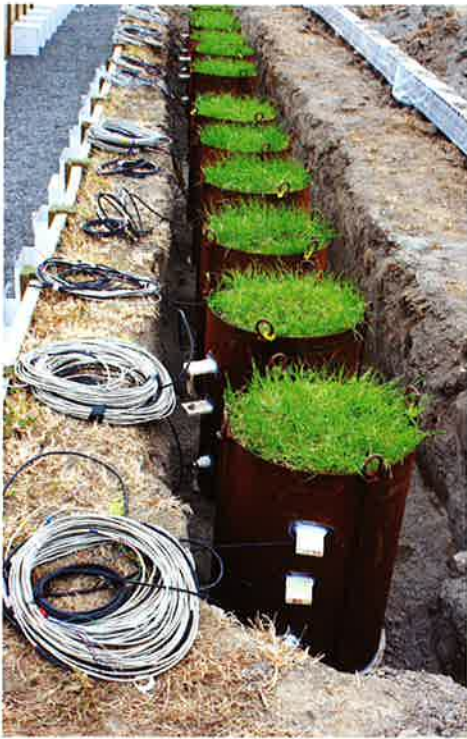
Figure 1 The lysimeter barrels placed into the trench at the new facility, showing cabling attached to sensors within the soil profile. Drainage is collected via a tube leading from the base to a collection vessel for later analysis.
