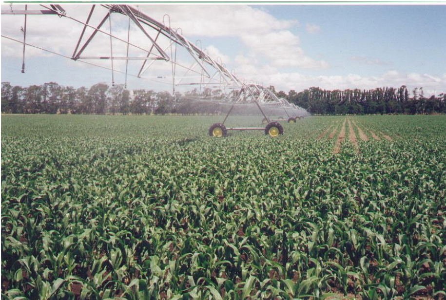
A lateral moving irrigator in use for sweet corn. Photo courtesy of Page Bloomer Associates.
