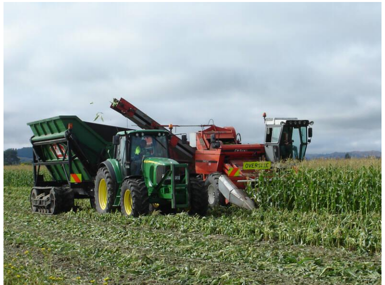
Harvesting in 2006. Note the tracked vehicle to carry the field bin. The tracks spread the load more evenly on the soil, reducing the potential for serious compaction problems for later crops.
