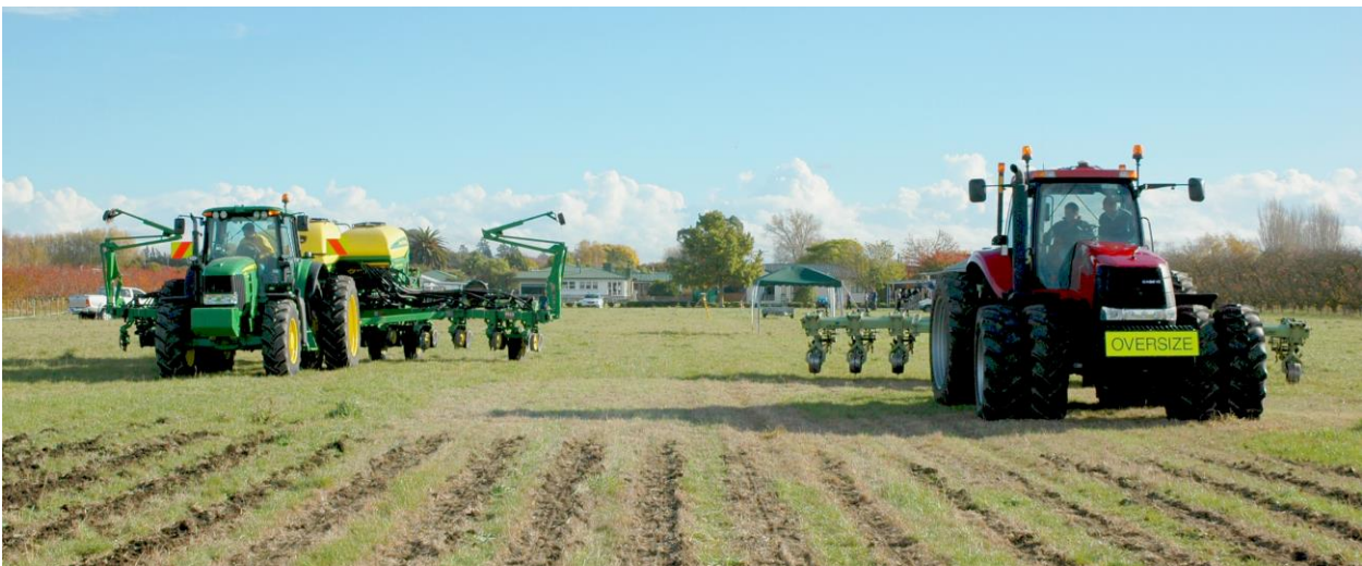
Strip tillage machinery reduces soil impact and together with other bout-matching equipment enables tramlining or controlled traffic farming to confine vehicle compaction.
